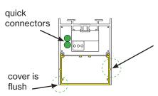
Cover must be fully engaged. You will feel a physical feedback and hear a "click" noise to confirm that the cover is engaged.
